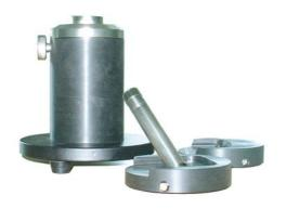
Artificial ear is designed to simulate human ear to test what human can hear.
